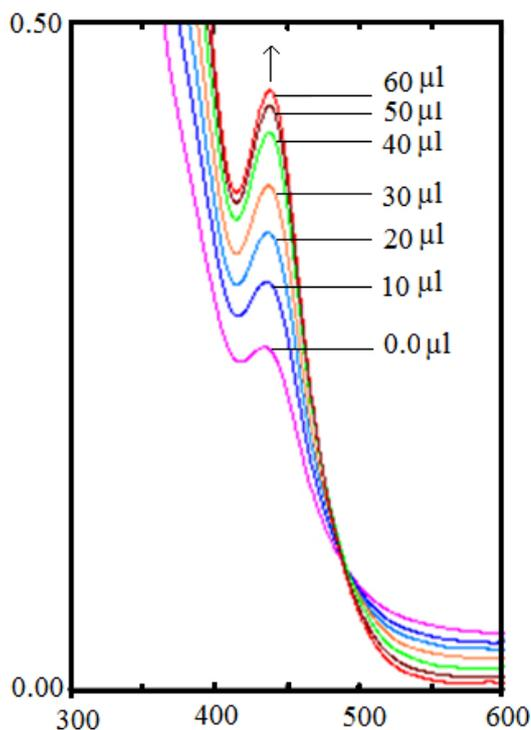
Fig. (3). Absorption spectra of complex 1 with increasing concentration of CT-DNA.
